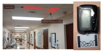
**Fig. 3** RFID system installed in the preoperative area. The system is placed above ceiling and unique tags are worn by staff surgeons
