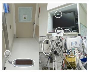
**Fig. 2** Installation of the smart OR system. Central computer where the data is collected from the sensors via 4G server (*top right*). IR sensor is also placed on the computer. Other images show the sensors installed in the OR. A camera in a 3D printed box (*bottom right*) is placed on the top of the ventilator bellows. Finally, two parallel pressure sensors protected by a plastic mattress placed at the doorstep (*left*)
