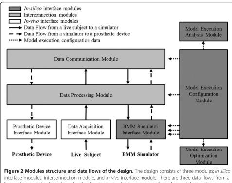
interface modules, interconnection module, and *in vivo* interface module. There are three data flows: from a live subject to a simulator, from the simulator to a prosthetic device, and from the model execution configuration module to other modules in order to set up the simulation environment with the user configuration parameters.
