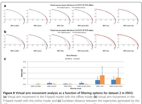
different simulation modes and the reference trajectory (averaged over 20 samples taken at 5 s intervals). The black dotted line shows the reference trajectories. The P-based model ran for 100 s of simulated time with the learning mode was turned off.
